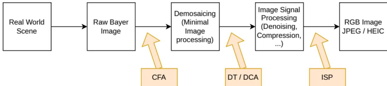
ISP "Image Signal Processing" Pipeline: JPEG and HEIC files from smartphones.
