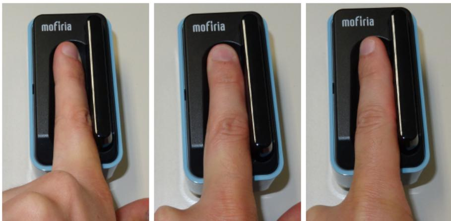
Figure: Finger rotation example using an off-the-shelf commercial scanner
