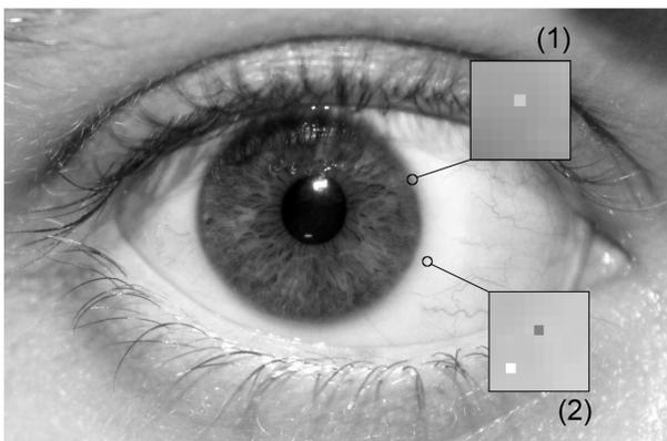
A *partially-stuck or hot pixel* (1) and two *stuck pixels* (2) in an iris image (enhanced for visualisation).
