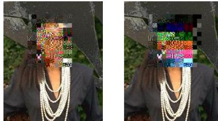
**Fig. 10** AC (left) vs. AC and DC encryption (right): When DC encryption is used, the RoI is extended visually on the right in some cases to compensate for the encryption-induced DC difference discrepancy. Original (uncropped) image from the *LIVE* reference picture set [35]
