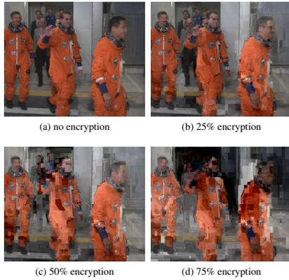
**Fig. 1.** Visual example of the sign encryption from the *crew* sequence with *randomaccess* structure and QP 21.
