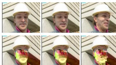
Figure 1: Examples for spatial and temporal drift: The first, second and tenth frame (from left to right) of the *foreman* sequence (top: original, bottom: encrypted) where one macroblock block row around the eyes in the first frame (left) has been encrypted.
