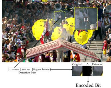
**Fig. 2** Extraction of a single watermark bit from a video under test.
