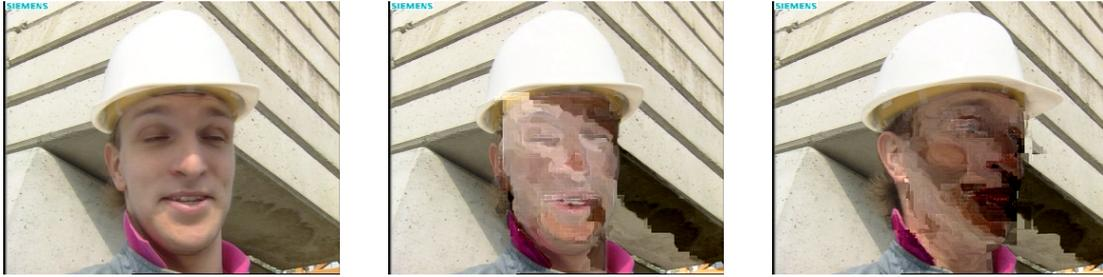
**Figure 1.3.:** Drift examples: In the original H.264-compressed frame (left), the face is encrypted (middle). The spatial drift on the collar and the concrete blocks in the background is due to inter-block dependencies between encrypted and unencrypted image regions. Future frames (right) exhibit additional temporal drift (e.g., the block beside the person's left eye) due to motion compensation in unencrypted image regions which use encrypted image regions as reference.
