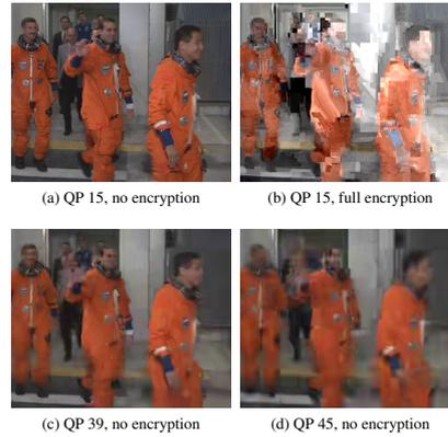
**Fig. 2.** Visual example of original and full sign encryption and different QP parameters.
