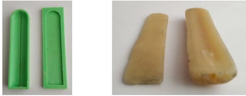
(a) 3D-printed molds to cast the artefacts (b) Top (l.) and bottom (r.) part consisting of beeswax
