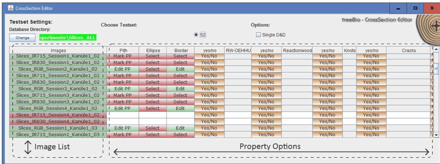
Figure 5.7: Overview of all CS-Images and wood properties for the selected testset.
