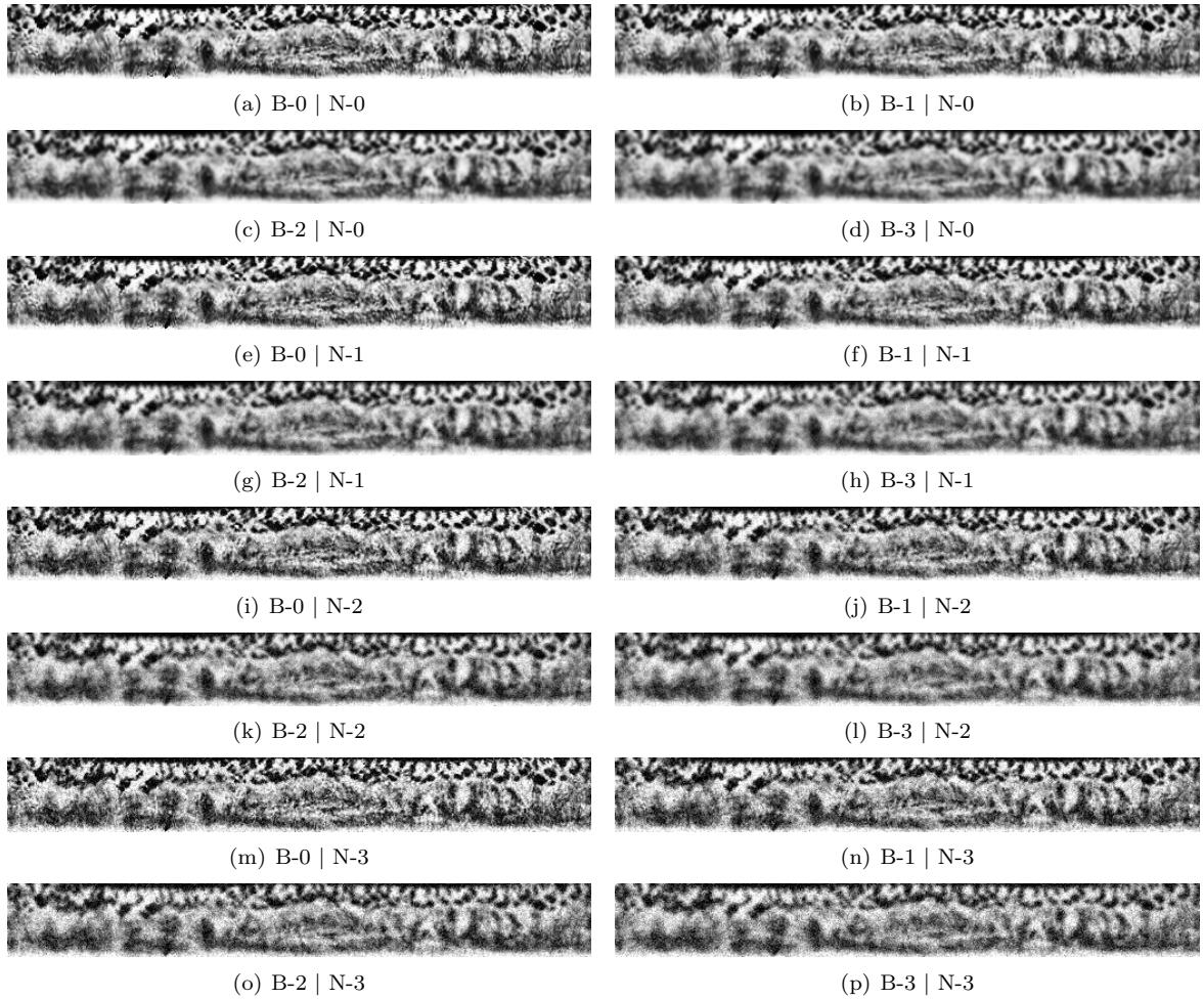
Figure 4: Signal degradation: (a)-(p) different intensities of blur and noise applied to a sample iris texture.
