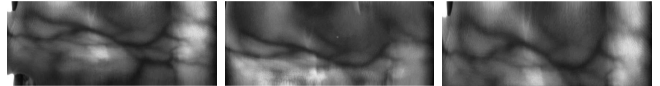
Fig. 2: ROI of sample images of the PLUSVein-FR after applying CPN. Left: palmar view ( 0^\circ ), middle: vein image captured at 45^\circ , right: 45^\circ artificially rotated version of the palmar image.
