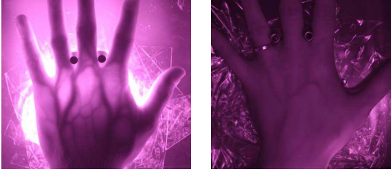
Figure 3. Example images of the the VeinPLUS data set. Left: transillumination, right: reflected light.
