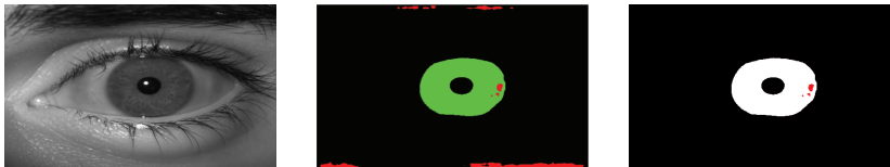
Figure 2: Sample iris image with P0 gaze-angle and its corresponding segmentation (green-color) and error mask (red-color) before (middle), and after correction (right), using the network trained on P0 images
