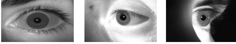
Figure 3: Sample iris images with P0 (left), N50 (middle), and P50 (right) gaze-angles
