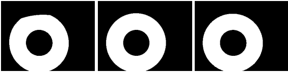
Figure 5. Segmentation masks of the expert ground truth [10], relative groundtruth seg(I_u^{(k)}) and an actual segmentation result seg(I_r^{(k)}) (f.l.t.r)
