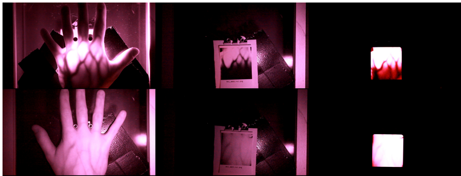
Figure: Example frames from NIR videos; top row: transillumination, bottom row: reflected light; left: real video frame, middle column: paper attack and right: smartphone attack, respectively. Captured with [3].
