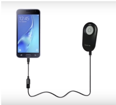
Recording device: Irishield device connected to a mobile phone (Samsung S8)
