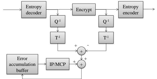
**Fig. 3.** Schematic transcoder architecture for RoI macroblocks (error accumulation): Differences between the encrypted and unencrypted values are accumulated in an error buffer.  $Q^{-1}$ : (inv.) quantization,  $T^{-1}$ : (inv.) transform, IP: intra prediction, MCP: motion-compensated prediction.
