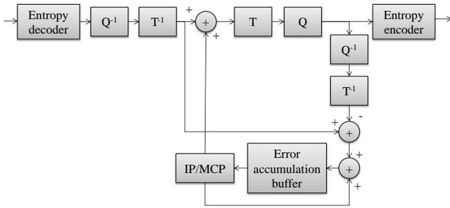
**Fig. 4.** Schematic transcoder architecture for macroblocks depending on the RoI (error compensation): The accumulated error is corrected approximatively by being considered in the prediction process. The abbreviations are the same as for Fig. 3.
