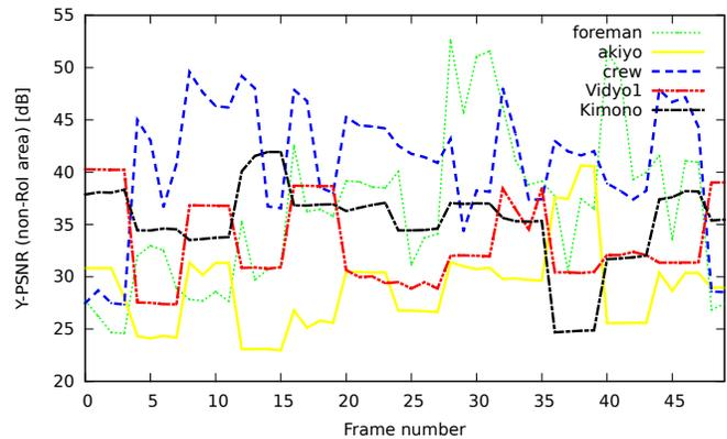
**Fig. 7.** Per-frame Y-PSNR outside the RoI for different sequences with QP 27 (first 50 frames): Spatial resolution has little to no effect on the quality degradation.
