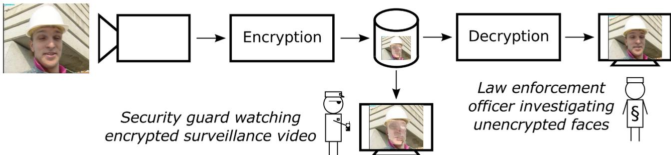
**Fig. 1.** Surveillance system use case: Images captured by a surveillance camera are encrypted and stored in a database. From there, the encrypted images can either be viewed directly or decrypted and used for legal investigations.
