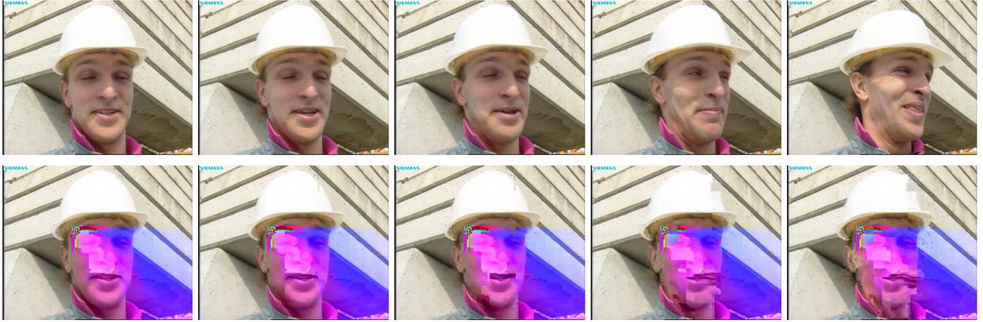
Figure 18: Example for temporal drift: The first, second, third, fifth and tenth frame (from left to right) of the *foreman* sequence where one block in the first frame (left-most) has been modified (as in figure 17). The top row shows the original frames, whereas the bottom row shows the frames with temporal drift (second from the left to right-most).
