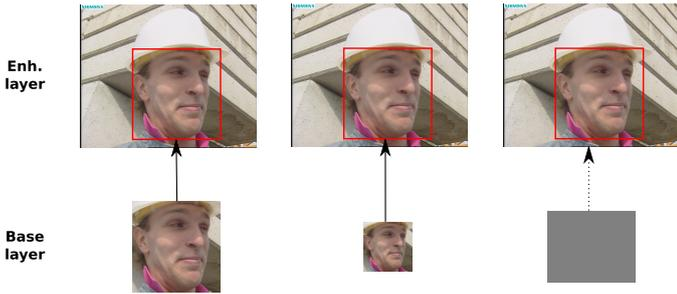
Figure 2: Alternatives to slice groups in the base layer: Left and middle: Extended spatial scalability; right: all-grey base layer
