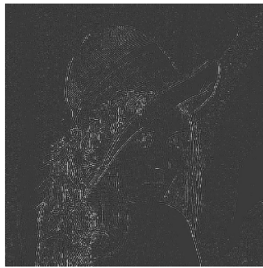
Fig. 5. First 20% encrypted, 2bpp, corrected concealment: PSNR 14.5dB, ESS 0.0
