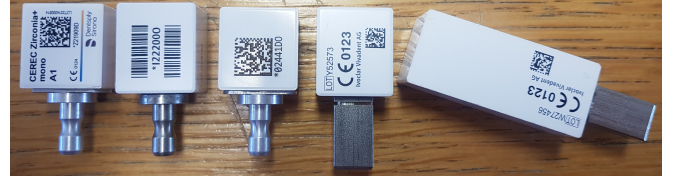
Fig. 1: Unprocessed Zircon Oxide Ceramic Blocks.
