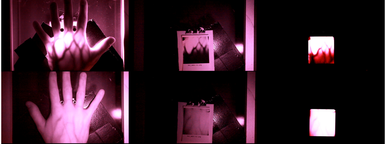
Figure 2: Example frames from NIR videos; top row: transillumination, bottom row: reflected light; left: real video frame, middle column: paper spoof and right: smartphone spoof, respectively
