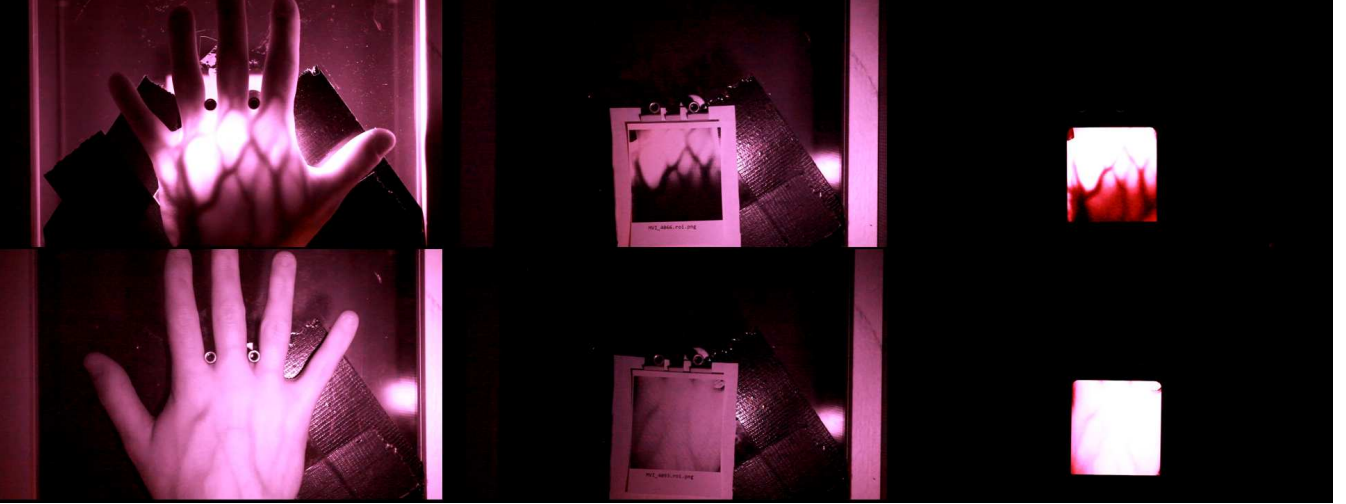
Fig. 2. Example frames from NIR videos; top row: transillumination, bottom row: reflected light; left: real video frame, middle column: paper spoofer and right: smartphone spoofer, respectively
