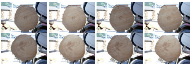
Figure 4: Testset One ( TS_1 ): Each row shows four CS-Images of a single log. The first two CS-Images illustrate the difference of capturing the log end with and without flash. The latter two images are taken after the log end was cross-cut, with and without flash.
