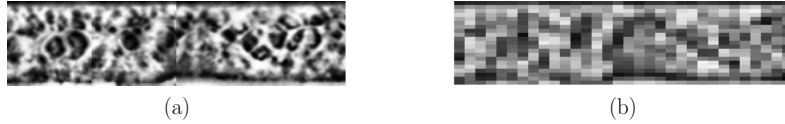
Fig. 2. Construction of the Archetype: (a) example of a preprocessed iris texture (b) the according archetype for 8 \times 3 pixel blocks. The mean grayscale value of each 8 \times 3 pixel block is assigned to the whole block.
