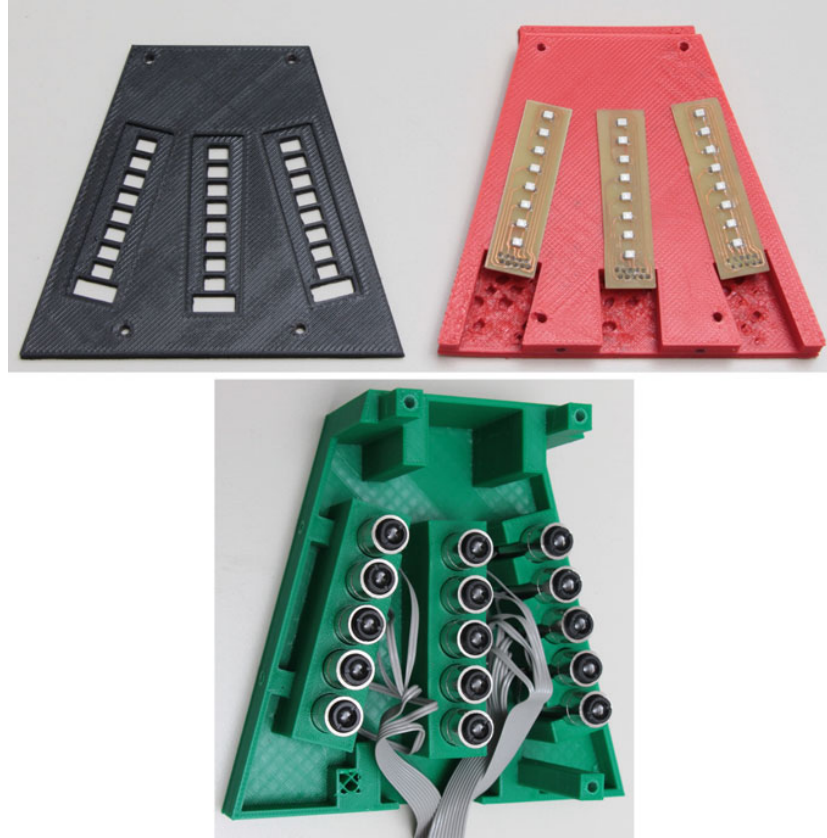
Fig. 3.8 Illuminator mounting bracket, top: LED version (two parts) + single LED stripes, bottom: laser version including the laser modules
