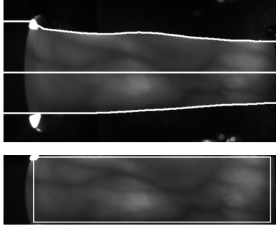
Fig. 8. ROI extraction - top: finger line detection. The straight line in the middle represents the center of the finger at which it is horizontally aligned. The top and bottom lines are the detected finger outlines which separate the finger from the background. The region between the lines is regarded as finger region. Bottom: the finger region is transformed to a fixed height. Afterwards the ROI, visualized as white square, of a fixed size is cut out.
