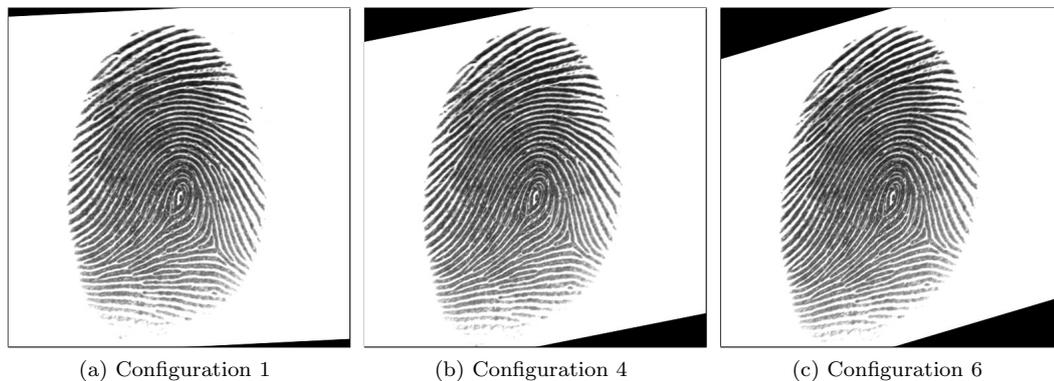
Figure 5.43: Examples for the *Affine Transformations – Shearing in Y-Direction* test, applied to an image from DB1 (ID 91.2).
